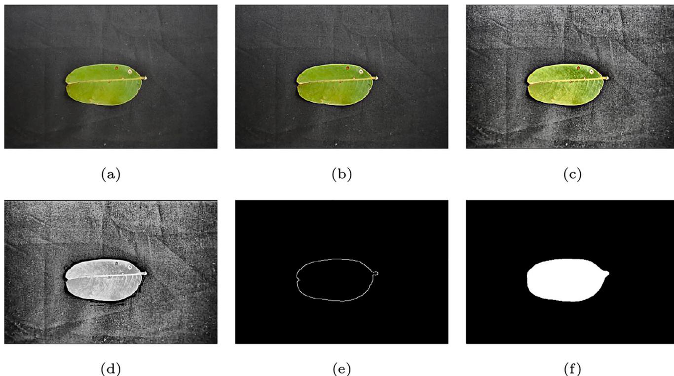
**Fig. 4.** Intermediate results of the background removal algorithm: (4a) Input image -  $I_{RGB}$  (4b) Sharpen Image  $I_{RGB}^S$  (4c) Adaptive equalization of the Lightness -  $I_{RGB}^H$ . (4d) Masked green channel -  $I_G^M$ . (4e) Canny edge detection applied on  $I_G^M - I_{Canny}$ . (4f) Final. (For interpretation of the references to color in this figure legend, the reader is referred to the web version of this article.) segmentation mask -  $Mask^F$ .
